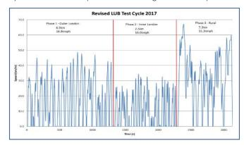
Coaches are to be tested using the 2017 LowCVP UK Coach cycle, consisting of an outer-city phase followed by a rural phase and ending with a motorway phase.
