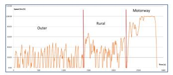
Heavy-goods vehicles shall be tested using the 2017 LowCVP UK HGV cycle (a combination of the Transport for London's AM Peak cycle and the World Harmonized Vehicle Cycle), consisting of an inner-city phase followed by urban, suburban and ending with a motorway phase.
