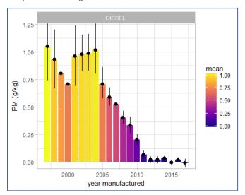
Ricardo's remote sensing data for Euro 5 and Euro 6 vehicles can also be used to ascertain whether substantial DPFs removals could be detected through corresponding increases in PM. Simulations have been run to estimate the effect of potential DPF removals, and results show that it might be possible to detect DPF removal at a 1% rate. However, for DPF removal rates from 5% and above it becomes much clearer that the removal can be detected.
