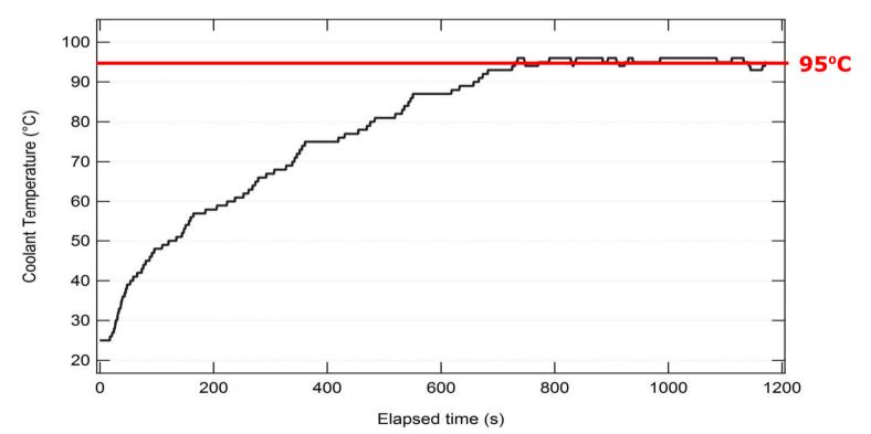
WLTC tests were conducted preconditioning the vehicle at constant speed ( $\sim$ 100km/h) until coolant temperature reached 95°C (stable temperature).
