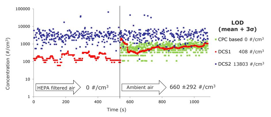
Even if the LOD of NM3 is higher that the LOD of Mod-NPET already at ambient PN concentrations both instrument shows the similar results
