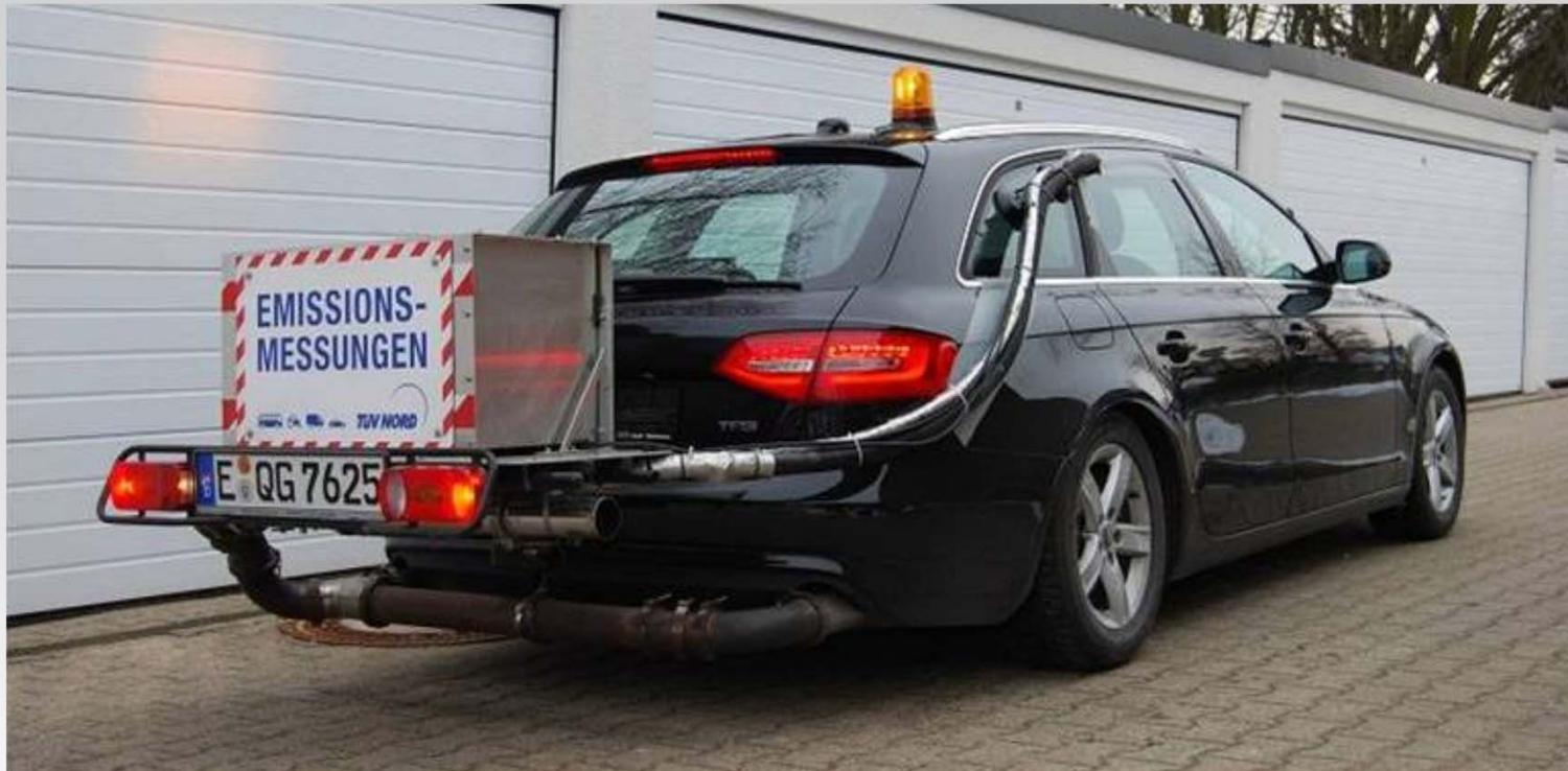
Portable Emission Measurement System (PEMS):
