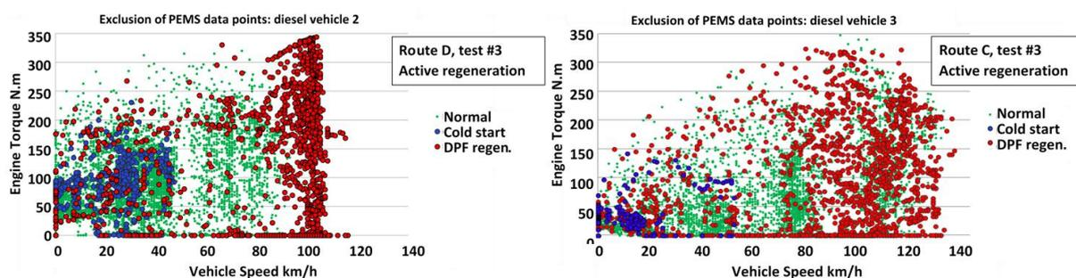
Figure 7: Effect of cold-start and DPF regeneration exclusions on gaseous emissions.
