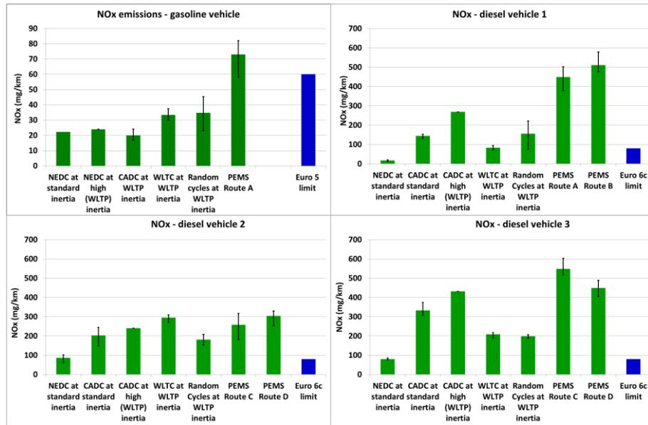
Figure 6: NOx emissions for the 4 vehicles, all tests.
