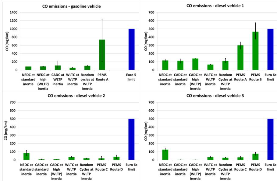
Figure 4: CO emissions for the 4 vehicles, all tests.
