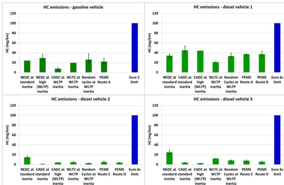
Figure 5: Total HC emissions for the 4 vehicles, all tests.
