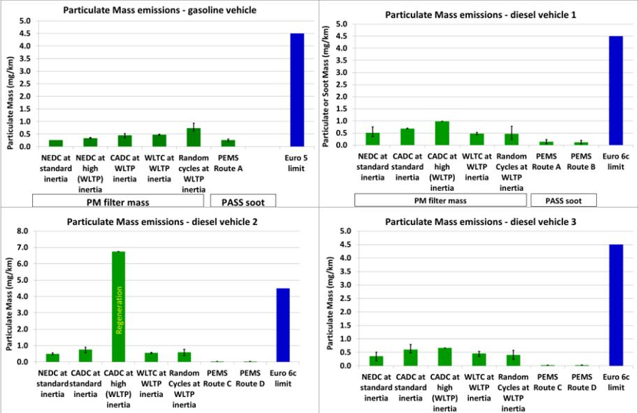
Figure 2: Particulate Mass (PM) emissions for the 4 vehicles, all tests.
