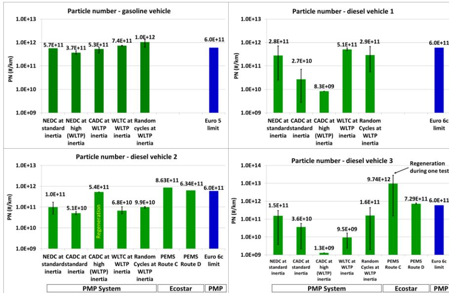
Figure 3: Particle Number (PN) emissions for the 4 vehicles, all tests.
