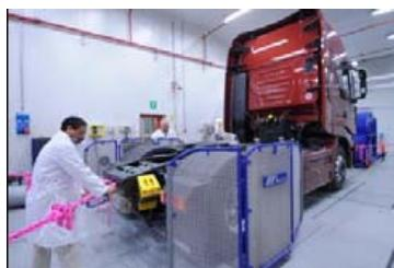
The new installation simulates wind drag, tyre/road friction and full drive cycles for real-life articulated lorries of up to 40 tonnes or 12 m-long buses.
