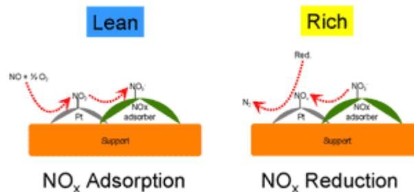
Figure 9: NO<sub>x</sub> adsorber system
