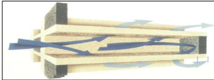
Figure 2: Exhaust gas flow through a wall-flow filter channel
