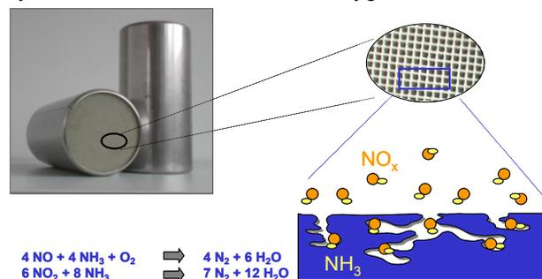
Figure 6: Selective Catalytic Reduction
