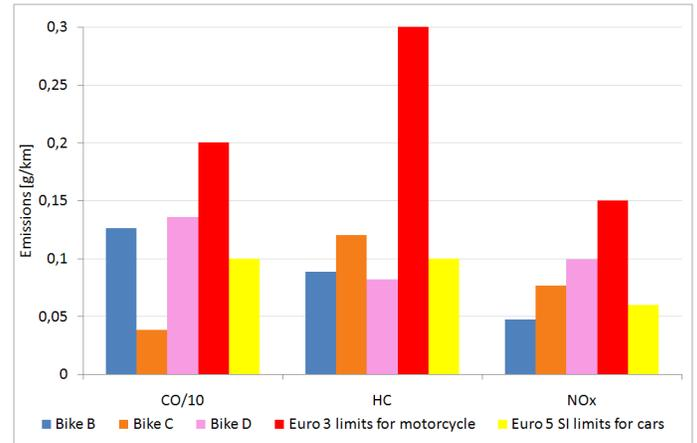
**Figure 15: Recalculated equivalent NEDC emissions from Euro 3 motorcycles**
