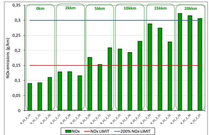
Figure 23: NOx emissions measured on Euro 3 cycle
