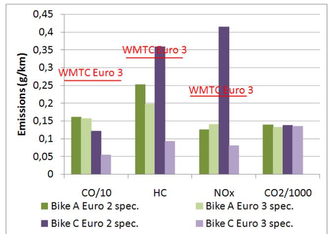
Figure 13: Euro 2 vs. Euro 3 bikes emissions on WMTC
