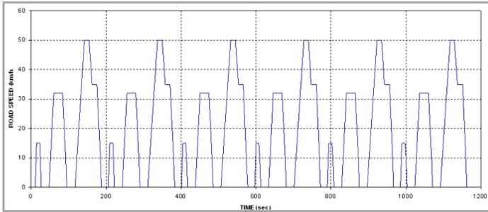
**Figure 2: "Euro 3" Emissions Test Cycle (<150cc)**
