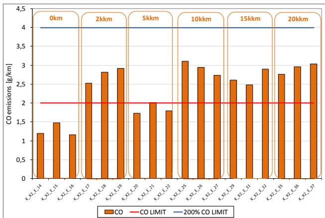
Figure 21: CO emissions measured on Euro 3 cycle
