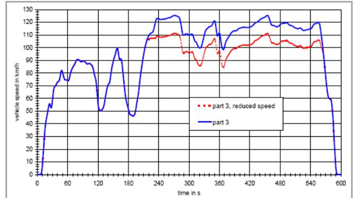
**Figure 5: WMTc part 3, for vehicle class 3**
