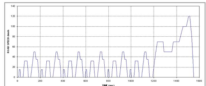
**Figure 1: "Euro 3" Emissions Test Cycle (≥150cc)**
