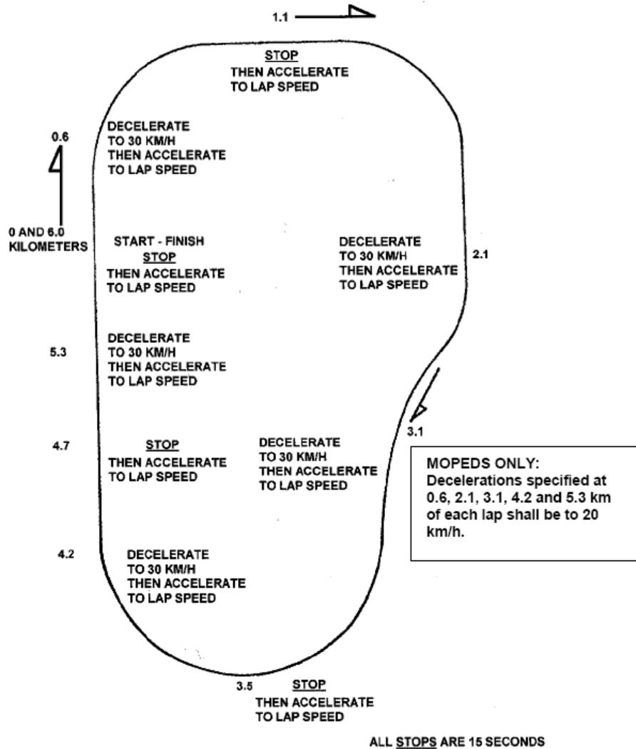
The durability cycle is composed of 11 cycles covering 6 km each.
