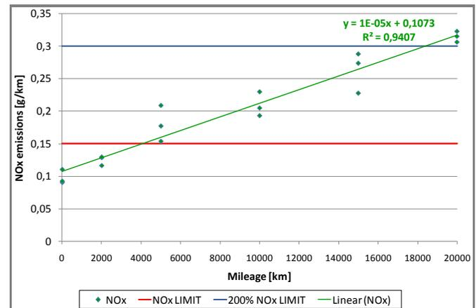
Figure 24: NOx emissions measured on Euro 3 cycle
