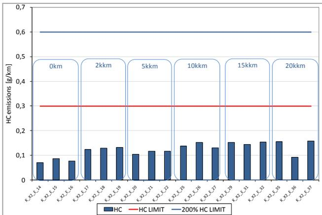
Figure 22: HC emissions measured on Euro 3 cycle
