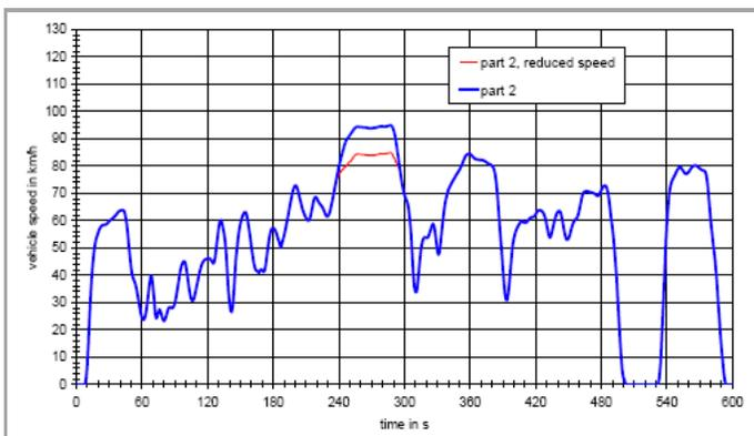
**Figure 4: WMTc part 2, for vehicle classes 2 and 3**
