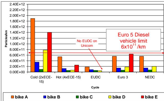
**Figure 16: Particle number emissions on European cycles**
