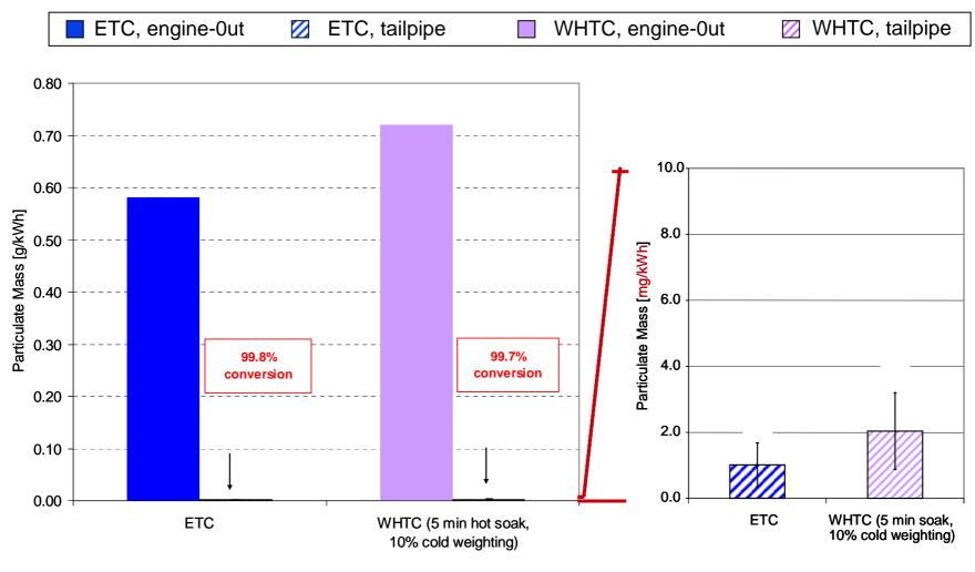
Measurements using partial flow (mini-dilution tunnel) system
