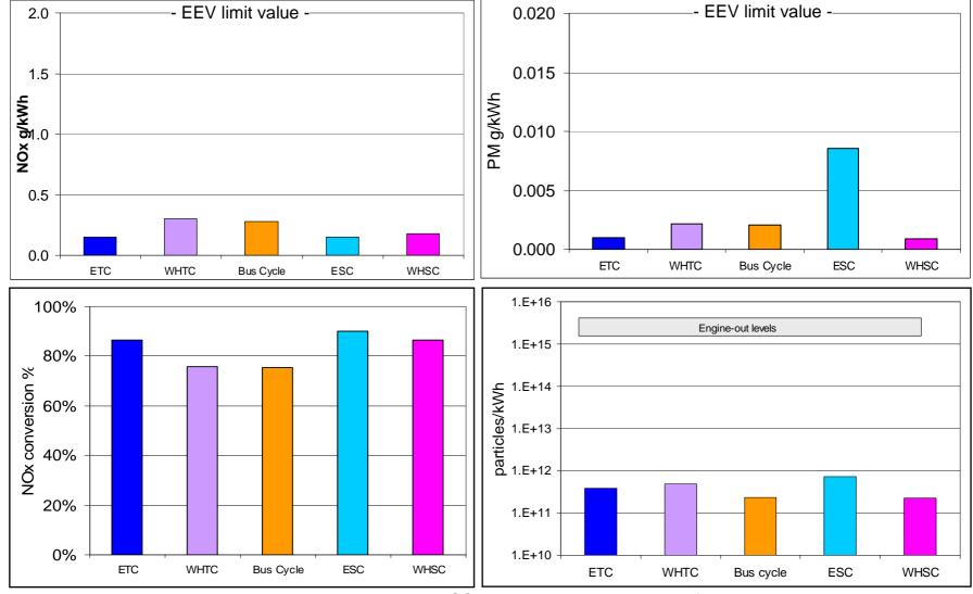
PM result on ESC appears due to desorption of low volatility materials in Mode 10.
