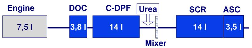
1m mixing length between injector and SCR face.
