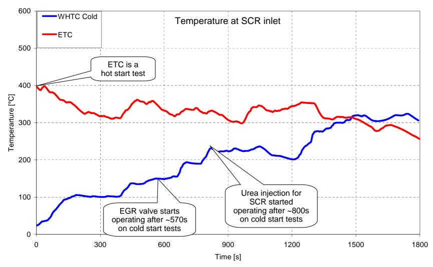
The results indicate that there is potential for further improvement of emissions on cold-start cycles through thermal management
