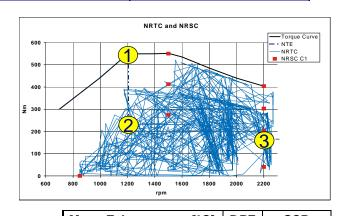
Mean Exhaust temp [°C] **DPF SCR COLD NRTC** 283 234 **HOT NRTC** 285 261 NRSC-C1 335 333 NRSC-D2 346 338 NRSC-F 323 342 NRSC-Fmod 326 342 NTE#1 411 378 NTE#2 388 343 NTE#3 300 319
