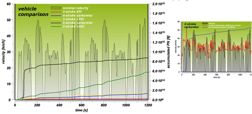
The overall pattern of PN emissions is similar to that for the ECE reg. 47 cycle. Again the -stroke carburettor moped shows a substantial number of particles near the start of the test, with a gradual increase thereafter.
