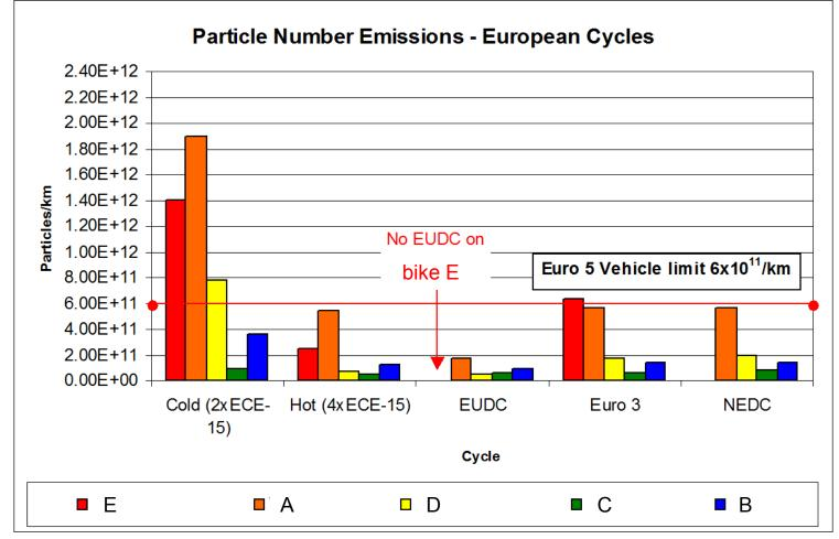
NEDC emissions from motorcycles calculated from cold start average (first two ECE-15 elements of the Euro 3 test), twice the average of the next 4 ECE-15 units and from the EUDC cycle average
