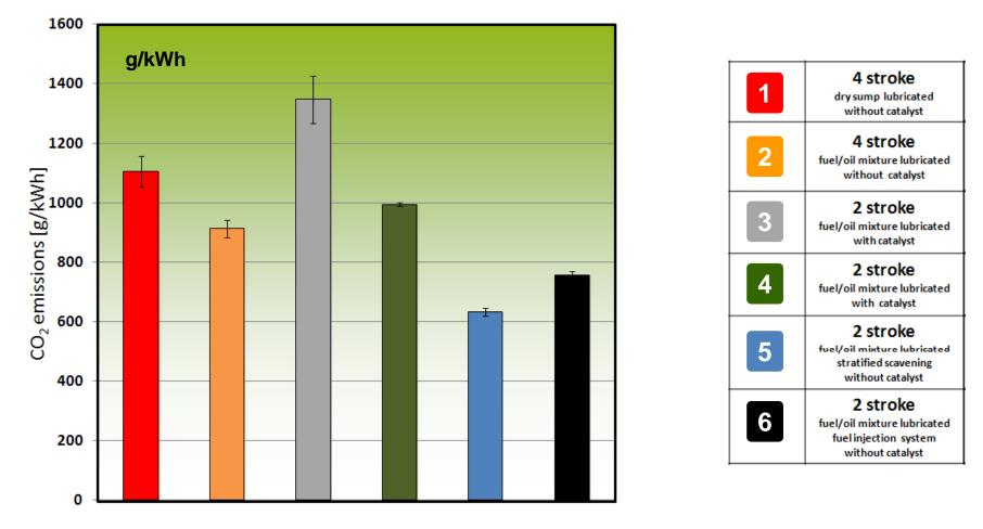
CO<sub>2</sub> emissions of engine N°3 are higher because of CO conversion by catalyst
