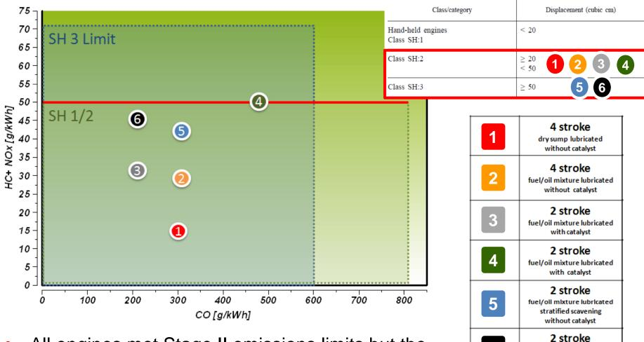
All engines met Stage II emissions limits but the low-cost model (N°4) is at the limit.
