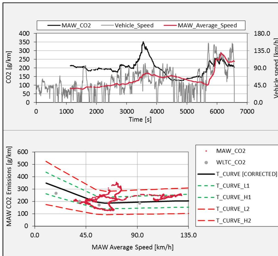
Figure 9: EMROAD analysis of the first RDE test
