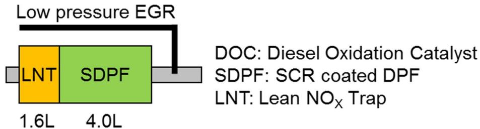
Figure 18: Main dimensions of the exhaust aftertreatment system in the simulation
