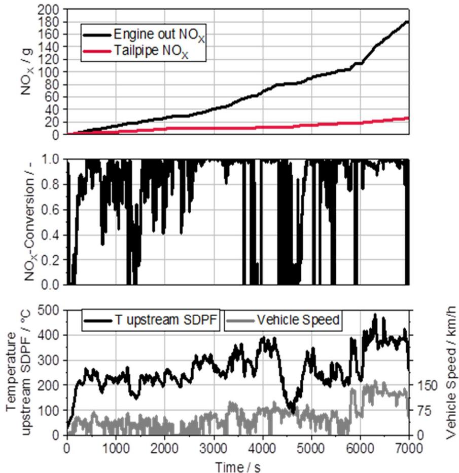
Figure 11: Results in RDE test with baseline calibration
