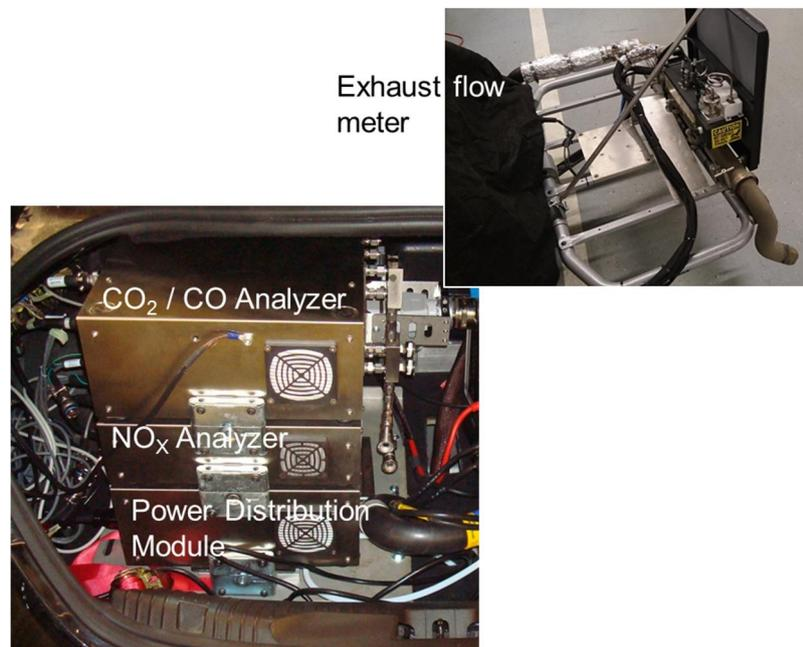
Figure 4: PEMS on the test vehicle
