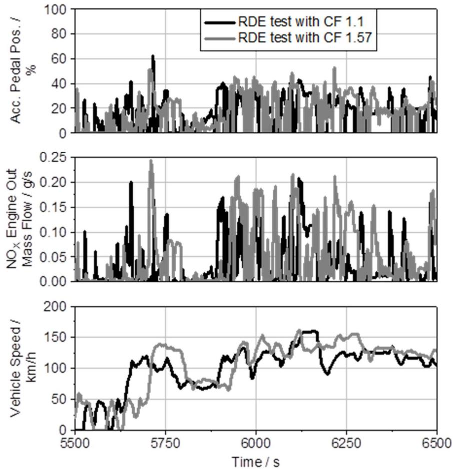
Figure 15: Detailed view of an extracted phase of both RDE tests with modified calibration
