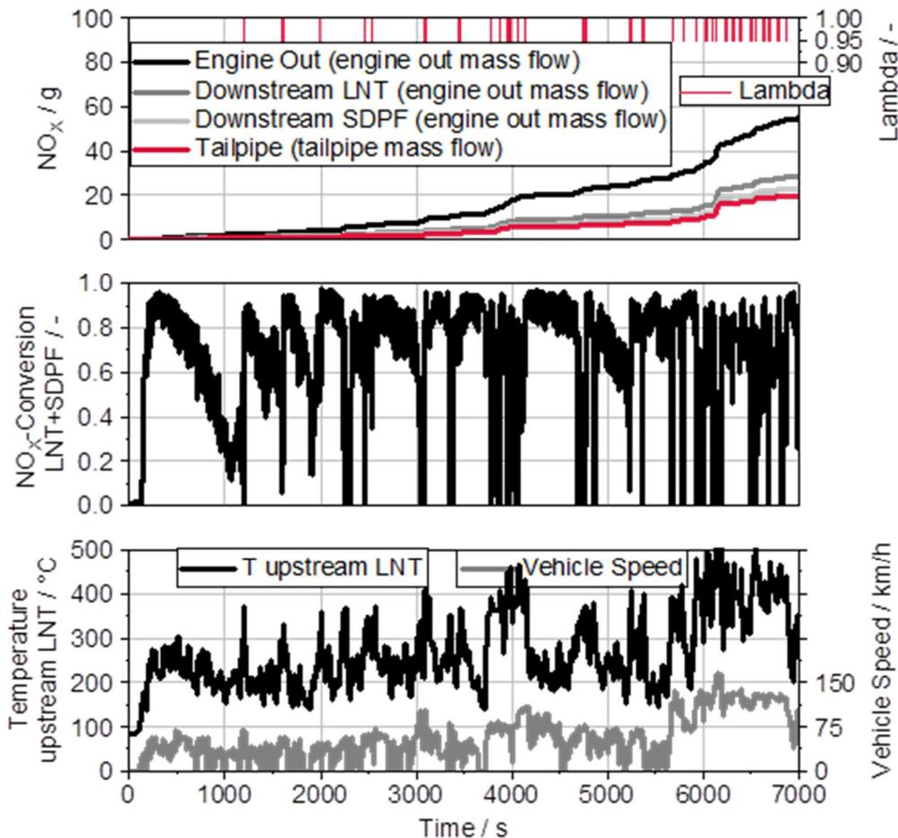
Figure 19: Simulated traces in the RDE test with LNT and passive SDPF
