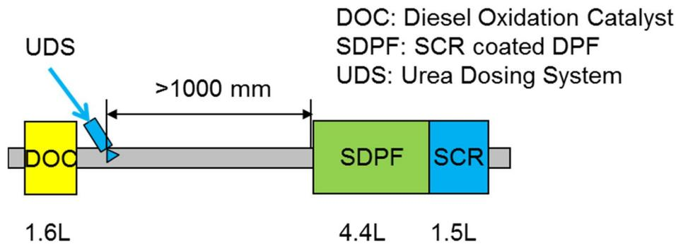
Figure 3: Main dimensions of the exhaust aftertreatment system on the test vehicle
