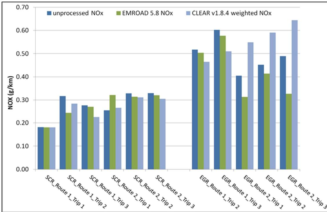
Figure 5: Comparison of the NO<sub>x</sub>-emissions with different evaluation methods [7]
