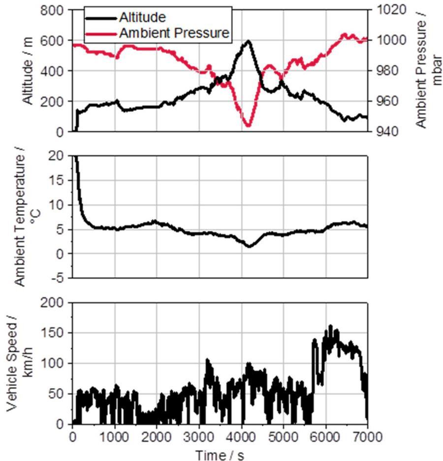
Figure 10: Boundary conditions of the RDE test with modified route
