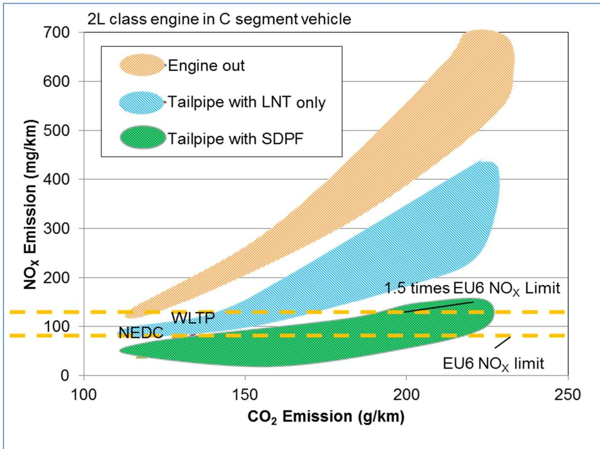
Figure 2: Exemplary increase of the NO<sub>x</sub> emissions depending on the driving cycle
