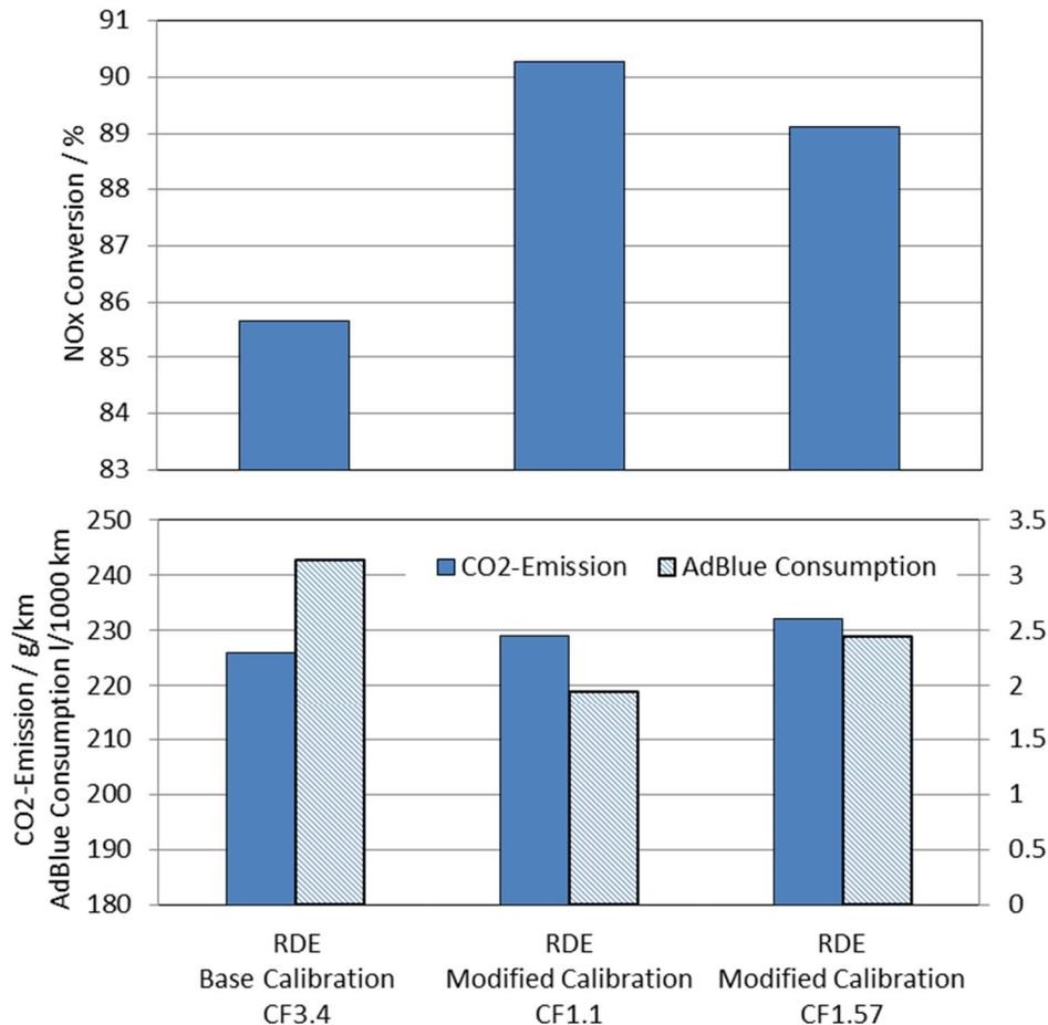
Figure 17: Comparison of CO<sub>2</sub>-emission and AdBlue<sup>®</sup> consumption in the RDE tests
