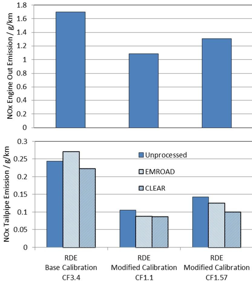
Figure 16: Comparison of the NO<sub>x</sub> emissions in the RDE tests
