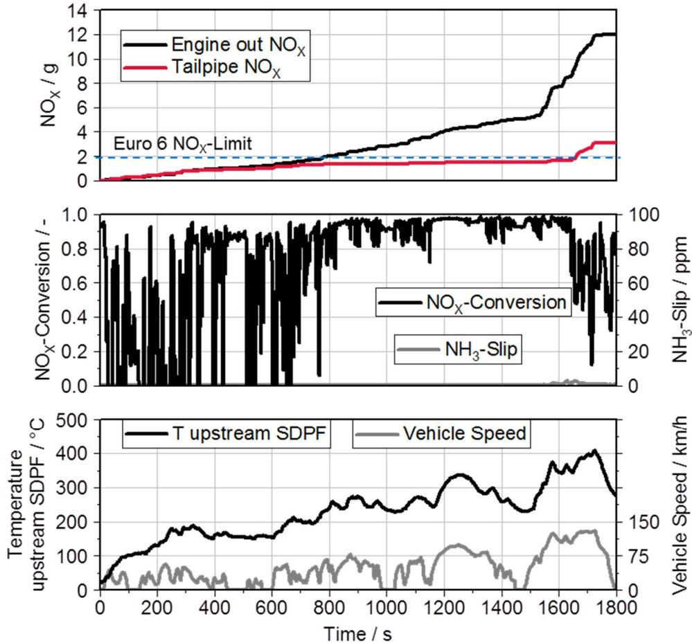
Figure 7: Results in WLTC with baseline calibration
