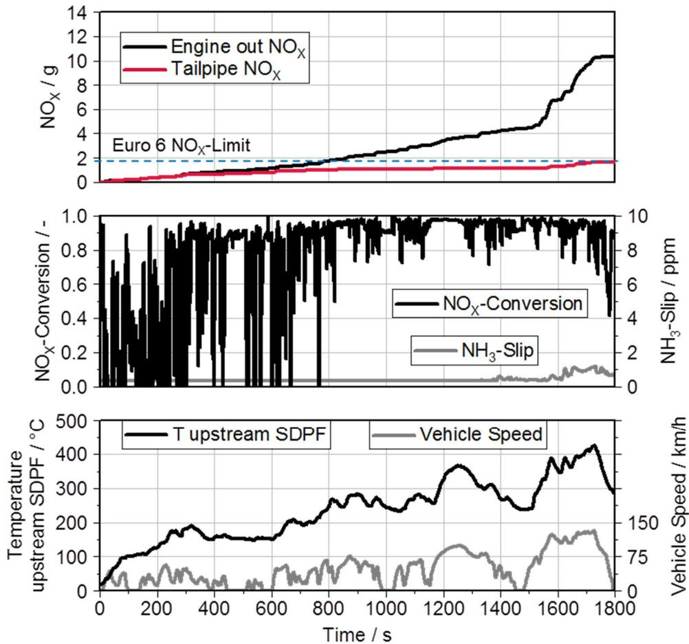
Figure 12: Results in WLTC with modified calibration
