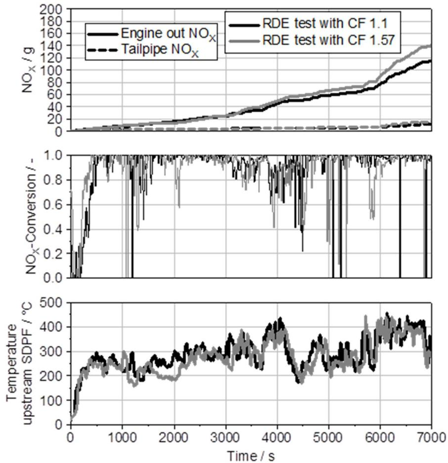
Figure 14: Results of the two exemplary RDE tests with modified calibration
