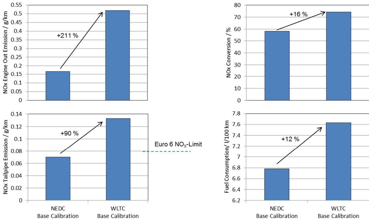
Figure 8: Comparison of the results in NEDC and WLTC with baseline calibration
