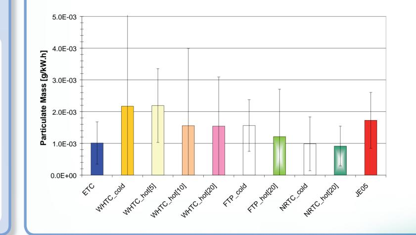
Comparison of average PM results using different methodologies shows <5mg/kWh in all cases
