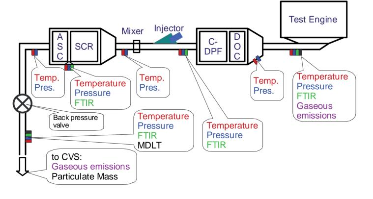
C-DPF – catalyst based Diesel Particulate Filter DOC – Diesel Oxidation Catalyst SCR – Selective Catalytic Reduction ASC – Ammonia Slip Catalyst
