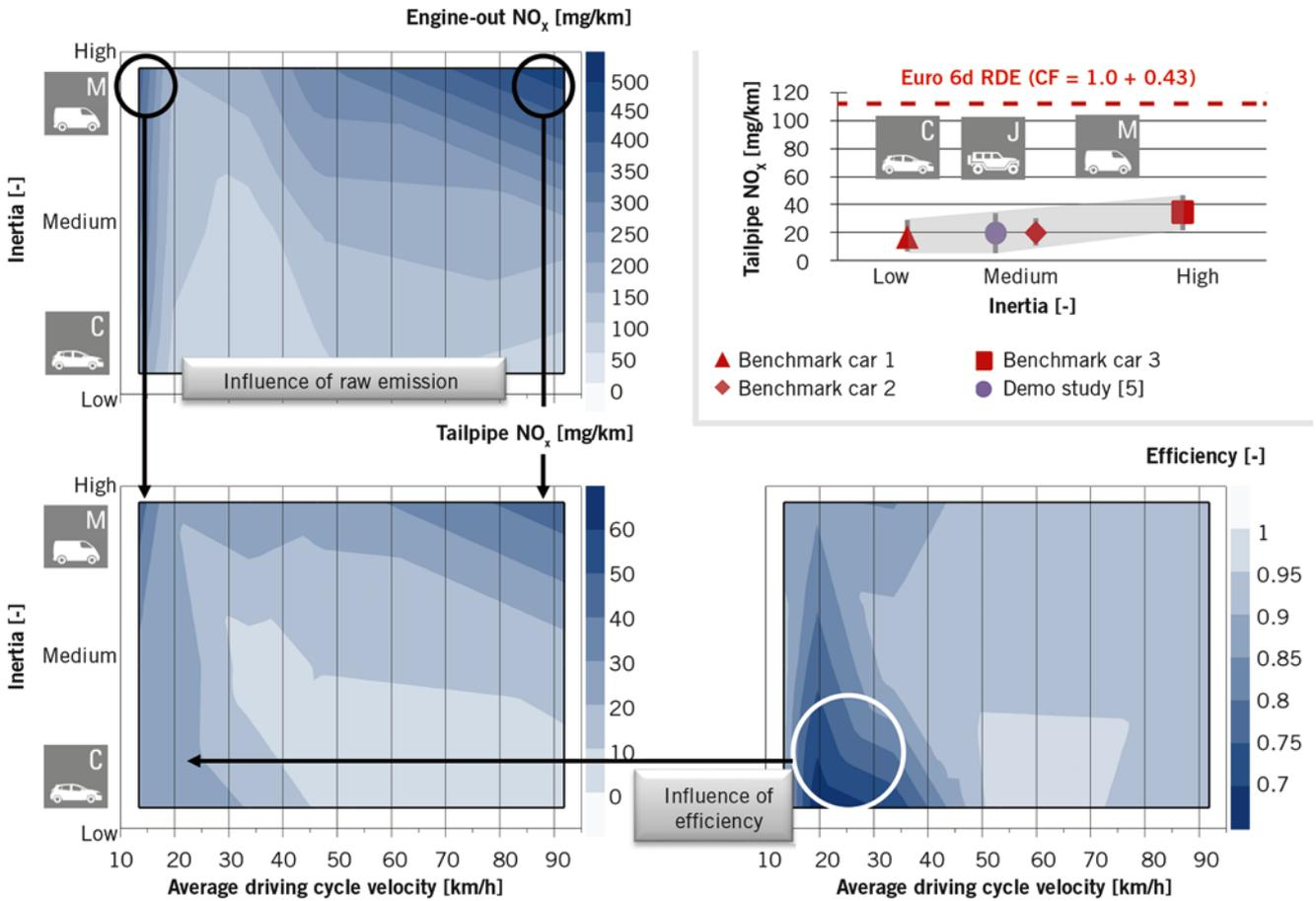
FIGURE 1 NO<sub>x</sub> emissions of Euro 6d and beyond with 2-l four-cylinder engines as function of weight and average cycle velocity under cold start conditions (© FEV)
