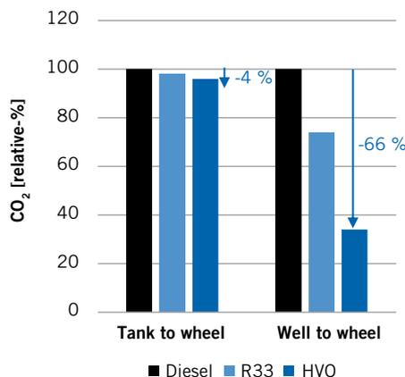
FIGURE 8 CO<sub>2</sub> emission for diesel and HVO in tank-to-wheel versus well-to-wheel consideration (© IAV)
