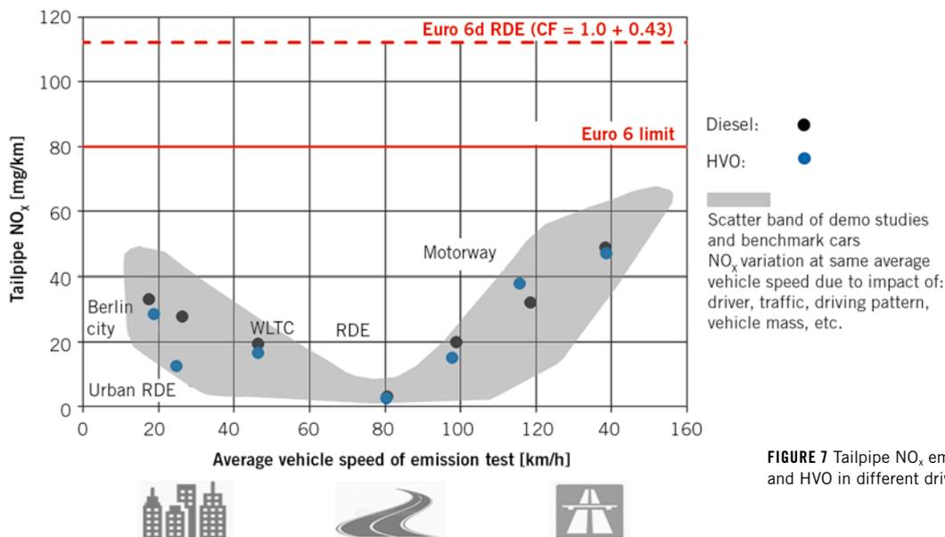
FIGURE 7 Tailpipe NO<sub>x</sub> emission for diesel and HVO in different driving cycles (© IAV)
