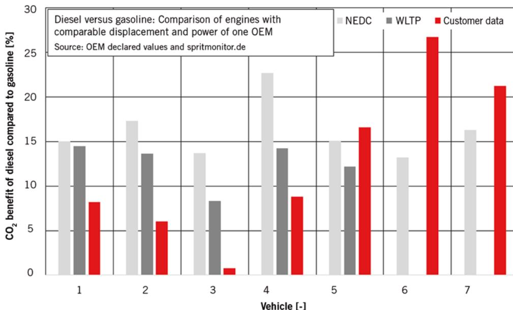
FIGURE 5 Inherent CO<sub>2</sub> advantage of diesel engines versus their gasoline counterpart for a specific vehicle model (© FEV)
