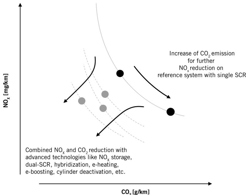
FIGURE 6 Schematic illustration of a possible combined NO<sub>x</sub> and CO<sub>2</sub> reduction (© AECC)
