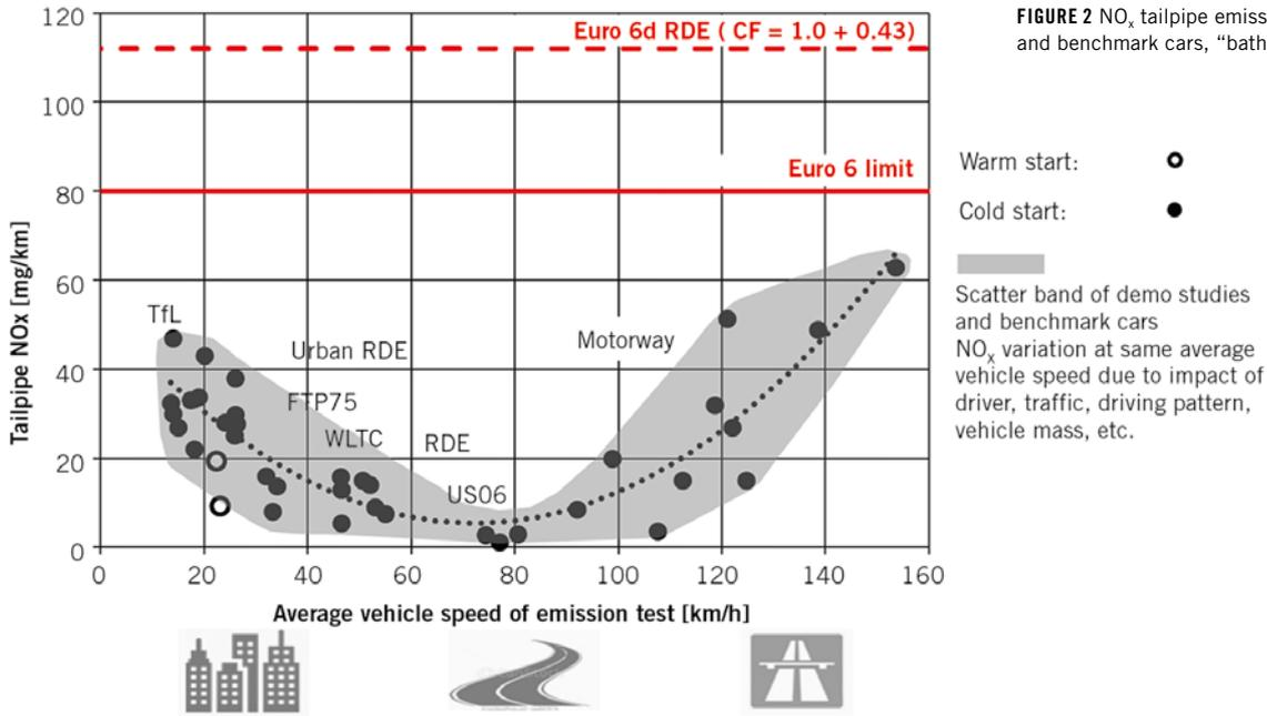
FIGURE 2 NO<sub>x</sub> tailpipe emission of various studies and benchmark cars, "bathtub-curve" (© FEV)
