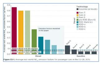
The results of emission-factor modelling indicate that the Baseline RDE scenario will reduce real-world NOx emissions of new Euro 6 diesel cars from 5.7 times the Euro 6 limit of 80 mg/km to approximately 4 times that limit. The Conservative RDE+ scenario is estimated to further reduce this emission factor to 2.1 times the Euro 6 limit.
