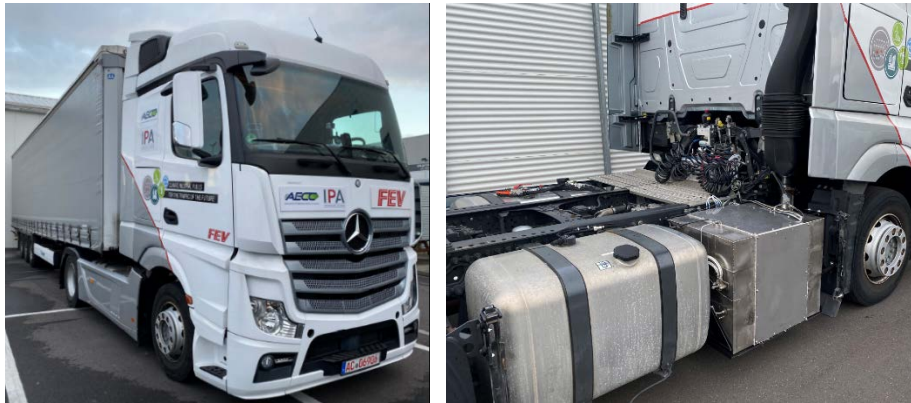
Figure 5: HD demo vehicle and the new ECT system installed.
