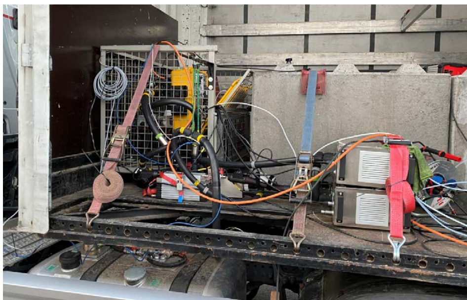
Figure 7: PEMS installed in the vehicle.
