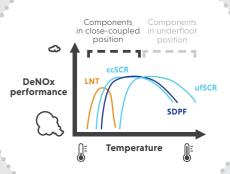
Achieving high NOx conversion rates, while preventing NH<sub>3</sub> slip was achieved via a model-based closed-loop control software.
