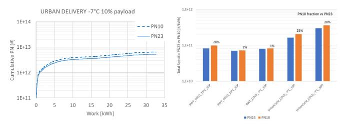
More PN data should be evaluated to judge emissions for combination of boundary conditions, including measurements of PN10. PN-slip during high-load operation in combination with pre-soot loading was for example not assessed.
