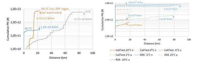
The variation in #/km over 2 orders of magnitude is impacted by a combination of effects, incl. ambient temperature, driving conditions, engine-out emissions and initial filter status. All diesel and gasoline tests were conducted with some amount of soot in the vehicle from on-road driving. No specific preconditioning was conducted to control the filter status in between tests. The order in which tests are conducted influences the results as well<sup>6</sup>.
