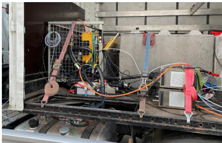
Fig. 2 PEMS installed in the vehicle.
