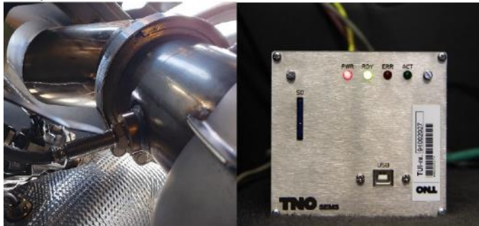
Figure 2: Smart Emissions Measurement System (SEMS). Left, emissions sensors in the tail pipe of an NRMM. Right, SEMS data recorder and transmitter to read, store and transmit sensor data, engine data and GPS data to a central server.
