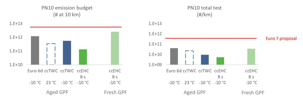
Note: RDE aggressive test results, 1.6 divider applied to data at -10 °C; the fresh GPF test is not a valid test according to the Euro 7 proposal
