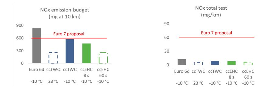
Note: RDE aggressive test results, 1.6 divider applied to data at -10 °C
