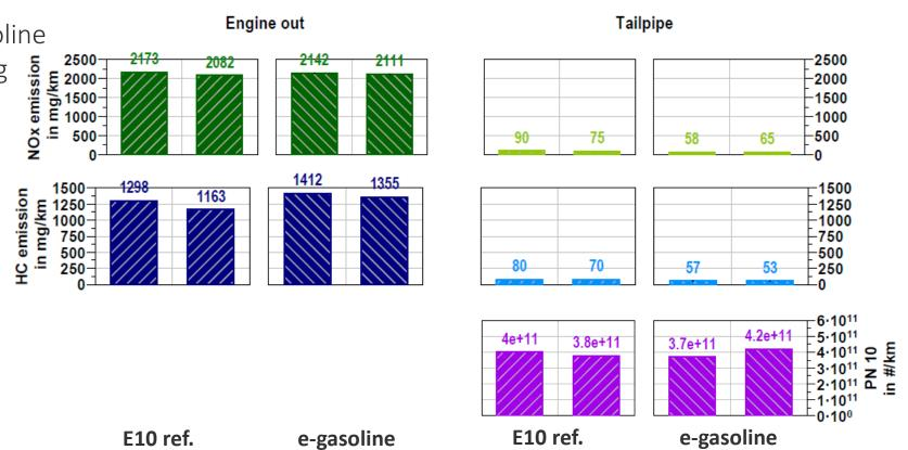
Note: RDE aggressive test results at -10 °C after 10 km (1.6 divider not applied), 2 test repeats on E10 reference fuel and e-gasoline
