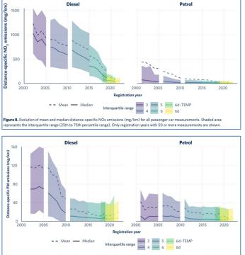
Figure 10. Evolution of mean and median distance-specific PM emissions (mg/km) for all passenger car measurements collected during the 2022 emission testing in Scotland. Shaded area represents the interquartile range (25th to 75th percentile range). Only registration years with 50 or more measurements are shown.
