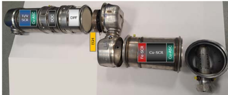
Figure 4: Modular emission control system
